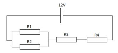
a) What is the effective total resistance of the network shown? Take the following as the resistor values:  $R1 = 3 \Omega$ ,  $R2 = 2 \Omega$ ,  $R3 = 4.3 \Omega$ ,  $R4 = 1 \Omega$ . (3 marks)
